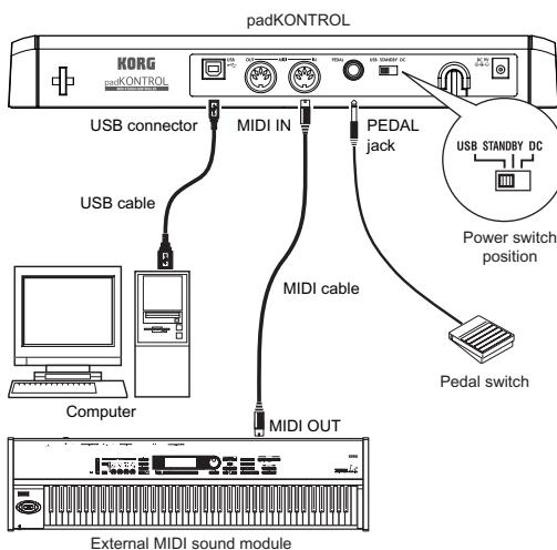
**note** The padKONTROL can function as a USB-MIDI interface. You can connect a MIDI sound module or other device to the MIDI OUT connector, and control the MIDI sound module from your computer.
